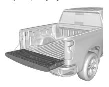
Press x2 twice on the remote key to open. See Remote Key Operation 14. If equipped with Keyless Access, the tailgate can be opened if the remote key is within 1 m (3 ft).
