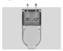
If equipped, trailering camera connectors are available in the bumper trailer receptacle in place of the four pin connector. The inside trailer auxiliary camera should be installed on the top left hand side (A) and the rear trailer auxiliary camera (B) should be installed on the top right hand side.
