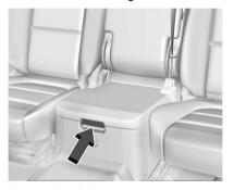
If equipped with front center seat storage, unlock with the mechanical key in the remote key, press the latch, and lift to open. See *Keys*
