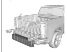
To close the inner tailgate with the primary tailgate closed, firmly push or pull it upward until it latches. Pull it back to be sure it is latched securely.
