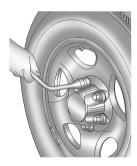
If the vehicle has wheel nut caps, loosen them by turning the wheel wrench counterclockwise.
