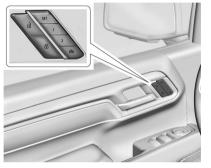
If equipped, the memory seat feature allows drivers to save their unique driving positions and a shared exit position. Other feature positions, such as power mirrors, may also be saved.
