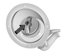
Use the fuel cap key to unlock the fuel cap then turn the fuel cap counterclockwise to remove. Fully insert and latch the fill nozzle, begin fueling.
