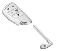
Press the button to remove the mechanical key. Never pull the mechanical key out without pressing the button.
