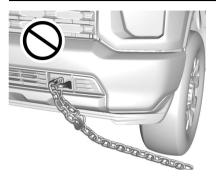
If equipped, there are recovery hooks at the front of the vehicle. Use them if the vehicle is stuck off-road and needs to be pulled some place to continue driving.
