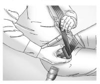
If the webbing locks in the latch plate before it reaches the buckle, tilt the latch plate flat to unlock.
