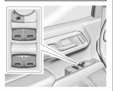
The power windows work when the vehicle is on, in accessory mode, or when Retained Accessory Power is active. See Retained Accessory Power (RAP) ⇒ 218.
