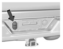
If equipped, the trailer wiring harness, with a seven-pin connector and a four-pin connector, is mounted on the vehicle's rear bumper.
