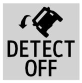
If equipped, the rollover detection disable button will be on the center stack in either the first, second, or third position.
