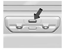
The MultiFrex (Chevrolet)/MultiPro (GMC) innertailgate may be equipped with an enable/ disable feature to prevent the inner tailgate from being opened when a hitch or other equipment is installed that could damage the inner tailgate.
