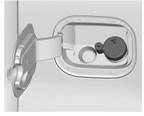
The vehicle has a locking fuel fill cover. Use the fuel fill cover key to unlock the cover. The key cannot be removed in the unlocked position. When reinstalling the fuel fill cover, be sure the arrow is pointing straight up.
