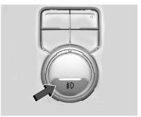
If equipped, the front fog light control is part of the headlight control located to the left of the steering column.
