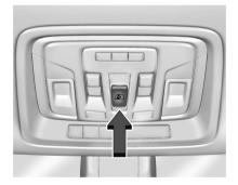
If equipped, the power sliding rear window works when the vehicle is on, in accessory mode, or Retained Accessory Power is active. See *Retained Accessory Power (RAP)* ⇒ 218. Press the switch to open the window and pull to close.
