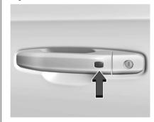
If equipped, the remote key must be within 1 m (3 ft) of the tailgate or door being opened or locked. Press the button on the door handle to open. See "Keyless Access Operation" in Remote Key Operation ▷ 14.
