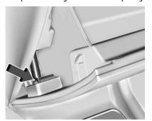
2. Push the dampener arm to the left until it releases the glove box.
