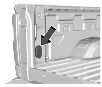
If equipped with the fifth-wheel/gooseneck trailer package, the harness connector is mounted on the inside of the pickup bed behind the rear wheel
