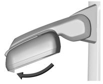
If equipped, grasp the mirror housing firmly and pull back in one motion, arching slightly toward the rear of the vehicle
